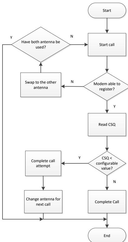
**Figure 39: Automatic antenna selection**
