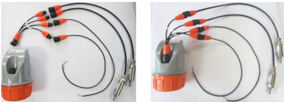
*Figure 44: Example cable assembly*
