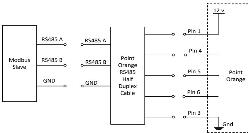
**Figure 19: Modbus RS485 Half Duplex connections**
