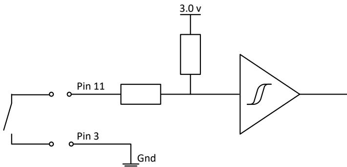
**Figure 6: Example DI connection circuit**
