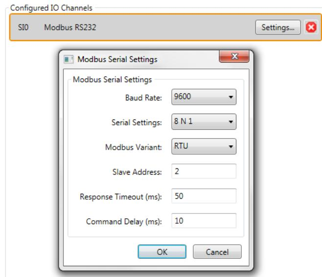
**Figure 21: Modbus configuration**
