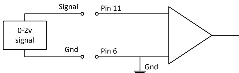
**Figure 15: Typical passive voltage connections**
