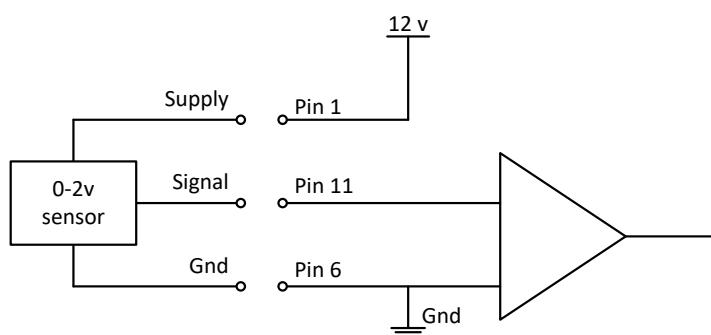
**Figure 11: Typical active voltage connections**
