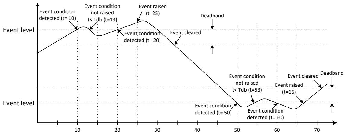
**Figure 35: Analogue level and time deadband example**
