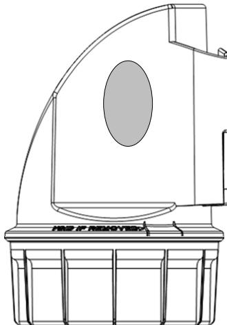
*Figure 28: Point Colour reed switch location*
