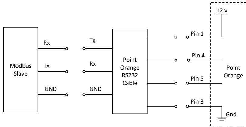
**Figure 18: Modbus RS232 connections**
