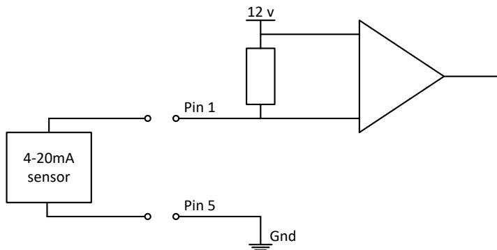
*Figure 9: Typical active loop connections*
