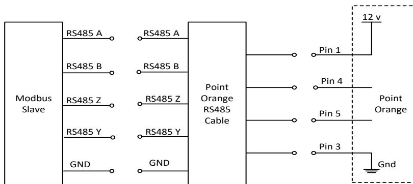
**Figure 20: Modbus RS485 Full Duplex connections**
