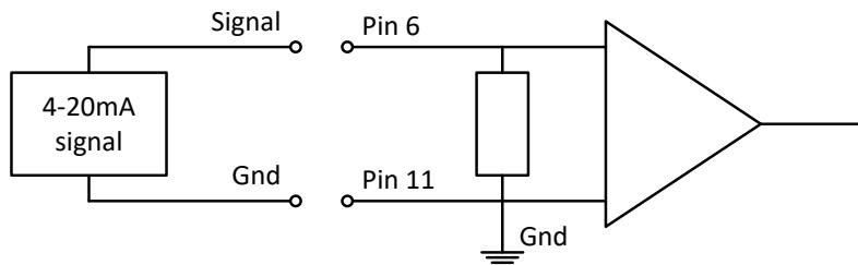
**Figure 13: Typical passive loop connections**
