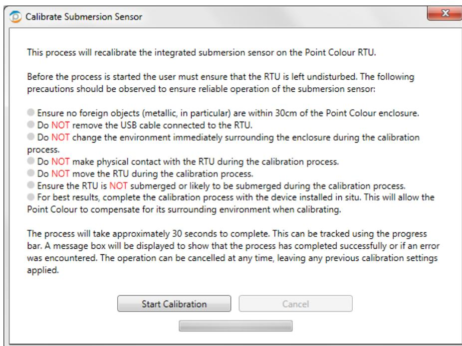
**Figure 30: Poco+ submersion calibration**
